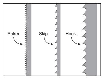
Figure 47. Raker, Skip & Hook tooth styles.
